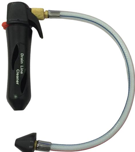
The Gel-clear Blockblaster Gallo Gun is a lightweight, portable tool designed for the quick and effective unblocking of condensate drain lines and other pipework. It utilises food-grade CO<sub>2</sub> cartridges to deliver a powerful blast, clearing blockages with ease.
