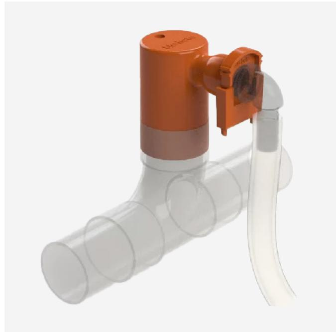
Designed for condensate pump discharge hose connections in the food retail cold chain, the CPH17 connector brings a water-tight seal to header drain connections stopping odour venting, backwash leaks and negative pressure in header drains. The connector prevents discharge hose pipes kinking with a 360 degree rotating hose barb, with quick release fitting.
